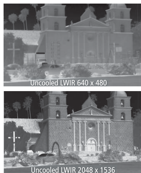
Figure 4. The dramatic resolution improvement using large format FPAs is illustrated in the images above that compare an uncooled LWIR image of the Santa Barbara Mission taken with a 640 x 480 pixel FPA (top) with an uncooled 2048 x 1536 pixel FPA (bottom).
