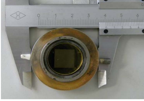
Fig. 8. FPA housed in a vacuum chamber with a diameter of 4 cm and a thickness of 1 cm.
