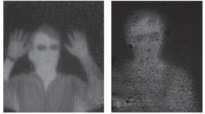
Fig. 13. Human's IR image detected by the FPA with (a) current design and (b) previous design.
