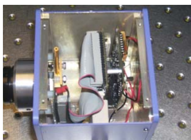
Figure 14. A schematic of the Alpha camera system, showing the 3 electronics boards located in the Camera unit (right) and camera
