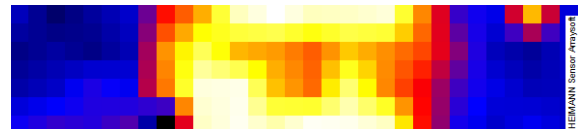
Fig. 6. Picture of the HTPA16x4 showing a person with glasses, taken and interpolated with the Heimann Sensor Arraysoft.
